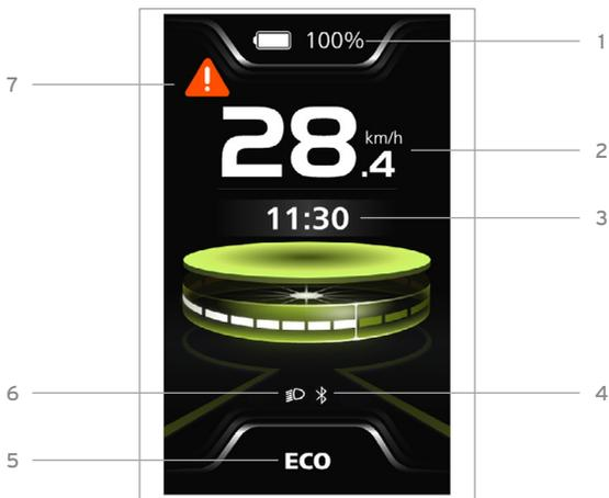
1. Indicator light for residual battery charge (%)
