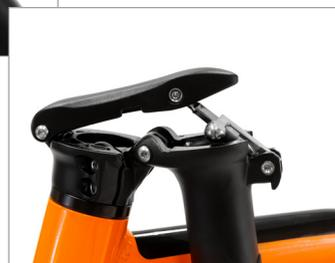
Pressing the lever locking device (A) present in the frame opening/closing mechanism towards the front of the electrically power assisted cycle, pull the lever (B) outwards until the locking pin can be removed from its seat.
