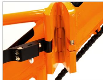
Fold the entire frame of the electrically power assisted cycle.
